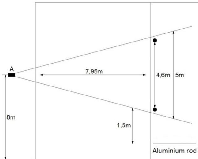
Figure 1. View of the measuring position on the lane in which the subjects moved (7.95 m) with the location of the camera (A) – in relation to the starting wall, the registered area (5 m), the maximum swimming speed area (4.6 m), and its distance from the rod (1.5 m)
