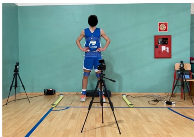
Figure 1. Testing area composed of OptoJump system and three GoPro cameras positioned 200 cm from athlete's standing position
