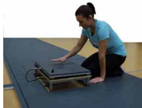
Figure 1. The experimental setup. Rhythm reproduction with the upper limb on a Kistler force plate (A)
