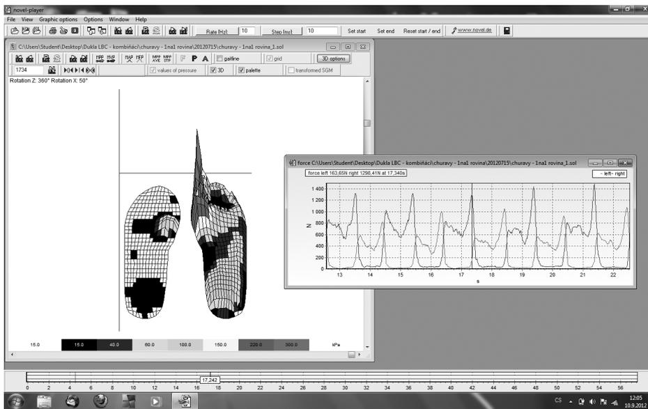
Figure 1. Example of the pressure distribution between the left (non-dominant) and right (dominant) leg observed using the Pedar system
