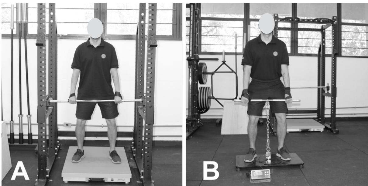
Figure 2. Isometric mid-thigh pull test. (A) Laboratory-based setup utilizing a force platform ('criterion'). (B) Portable custom-made setup utilizing a load cell ('low-cost')
